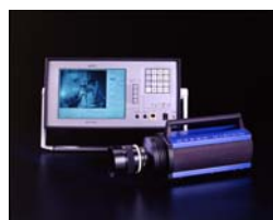
Fig 4: Developed for materials testing and development: the HPV-1 high-speed camera can capture 100 images at one million frames per second.
