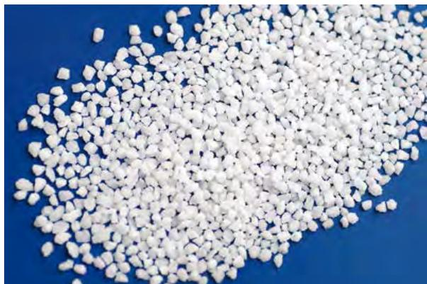
High salt concentrations generally present a problem for TOC analysis. These salts can crystallize in the combustion system and lead to higher maintenance needs.
