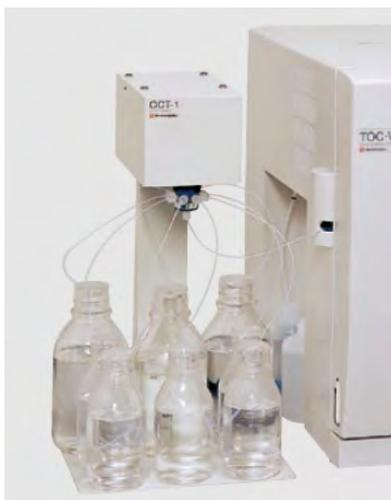
The autosampler OCT-1 has a big advantage for the measurement of aggressive matrices, because its parts are done of Teflon.
