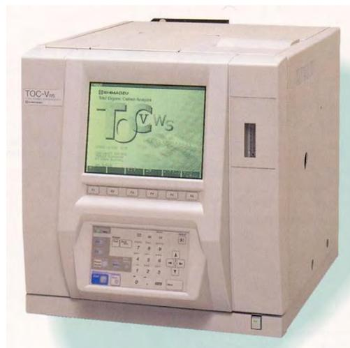
Its core technology is the powerful oxidation applying a combination of sodium persulfate and UV oxidation at 80 °C. This ensures that all dissolved carbon compounds are converted to CO<sub>2</sub>.
